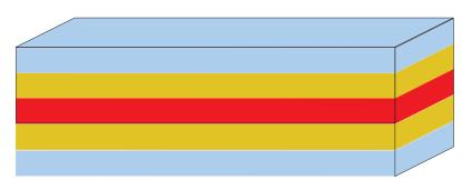
PET Release Film (Light Release) 0.036mm Modified Solvent Acrylic Adhesive (Neutral) PET Carrier
